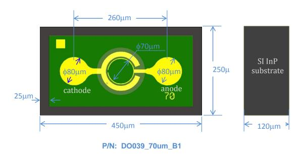
Attention: InP brittle material and electrostatic sensitive device, observe precaution for handling.
